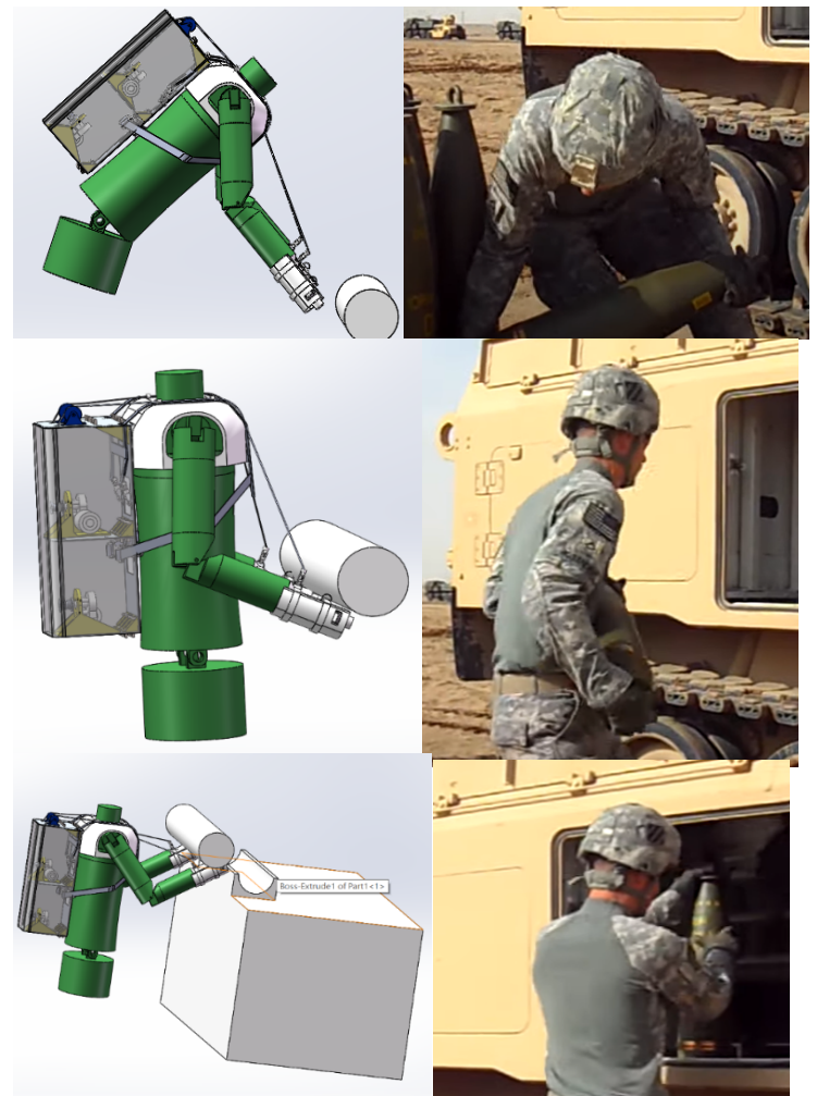
Figure 4: Cable Assisted Arms Movement Diagram
